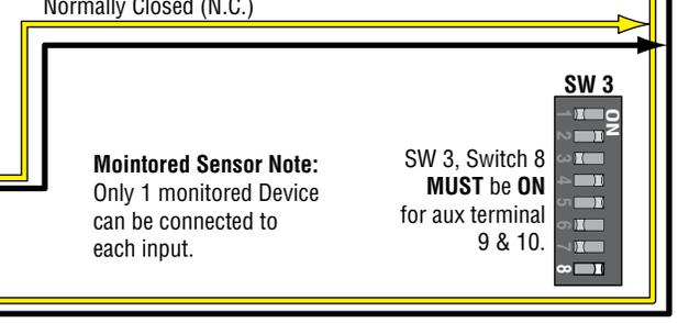
**Monitored Sensor Note:** Only 1 monitored Device can be connected to each input.
