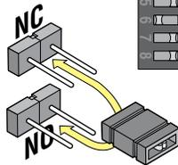
24-volt DC magnetic lock power is provided constantly except when the gate is **opening** or **open** (Normally Closed function). 1 Amp Max.
