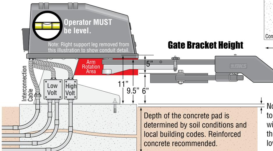
Note: If allowed by local codes, the top of the concrete pad can be flush with ground level, which will allow the gate bracket to be mounted lower on the gate.
