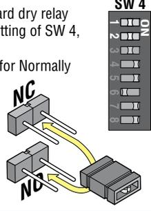
24-volt DC magnetic lock power is provided constantly except when the gate is **opening** or **open** (Normally Closed function). 1 Amp Max.
