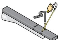
**2. In the event of a primary (AC) power failure and a back-up system (DC) power failure** (low charged or dead batteries for example), the system must have a release system to allow the gate to be **Manually Operated**.
