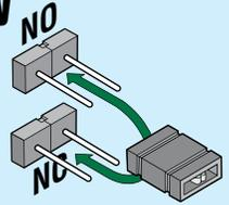
Dry relay contacts (terminals 16-17) can be set for Normally Open (NO) or Normally Closed (NC) operation by placing the relay shorting bar on the N.O. or N.C. pins respectively. (Standard shadow loop function, NO)
