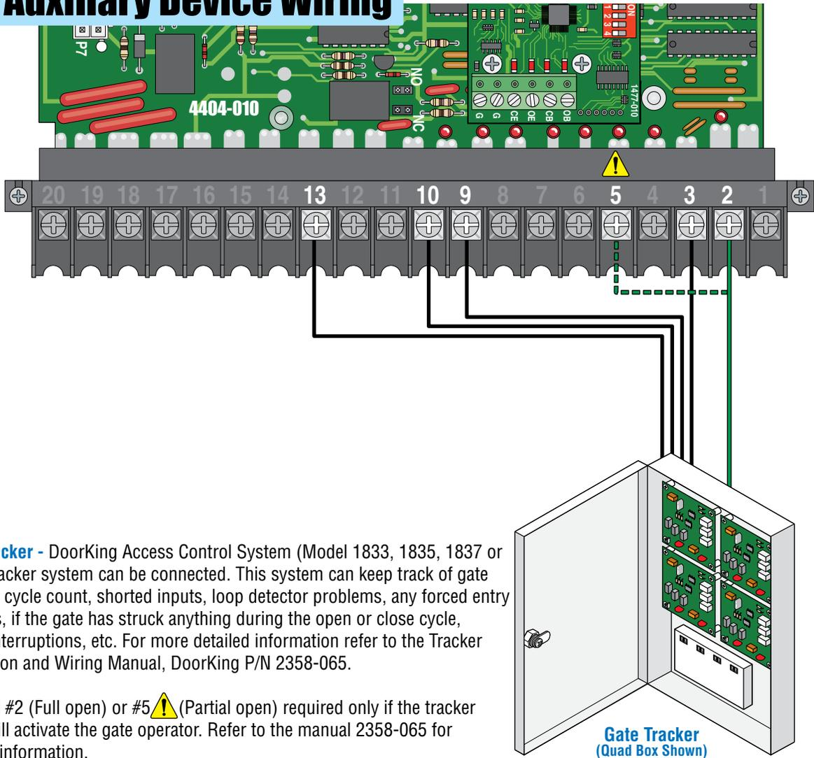
**Gate Tracker** - DoorKing Access Control System (Model 1833, 1835, 1837 or 1838) tracker system can be connected. This system can keep track of gate operator cycle count, shorted inputs, loop detector problems, any forced entry attempts, if the gate has struck anything during the open or close cycle, power interruptions, etc. For more detailed information refer to the Tracker Installation and Wiring Manual, DoorKing P/N 2358-065.
