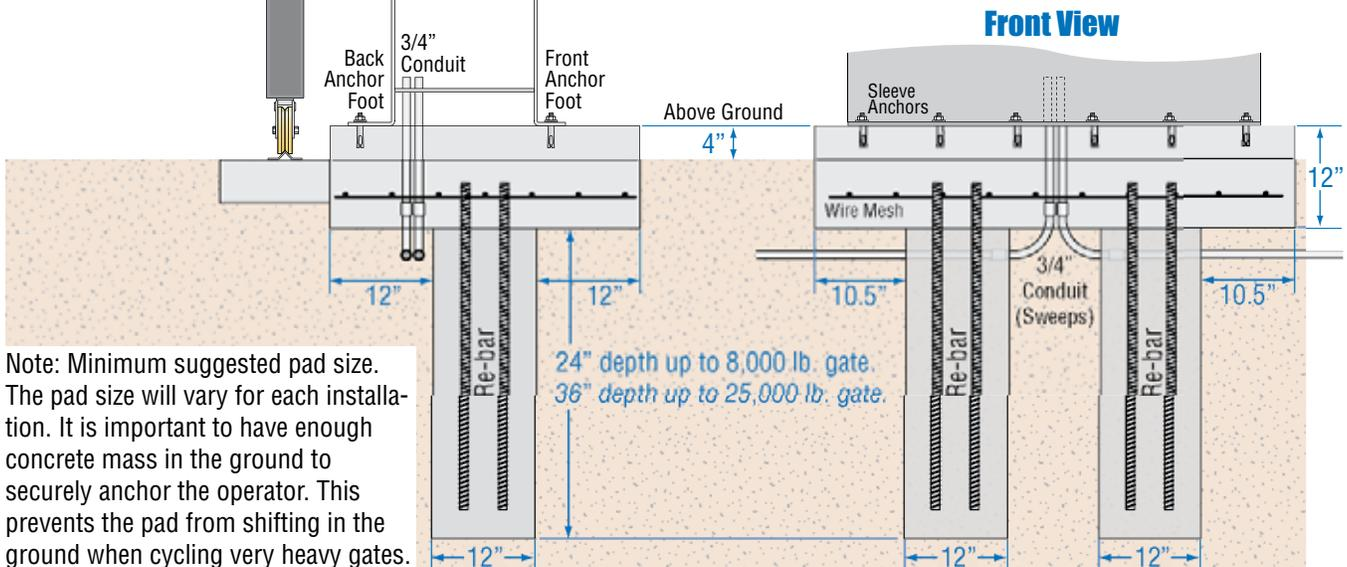
Note: Minimum suggested pad size. The pad size will vary for each installation. It is important to have enough concrete mass in the ground to securely anchor the operator. This prevents the pad from shifting in the ground when cycling very heavy gates.
