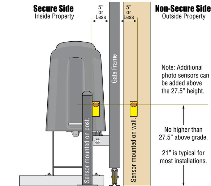
Photo sensors may be installed on either side of gate frame, as close as practical to the gate but no further away than 5".
