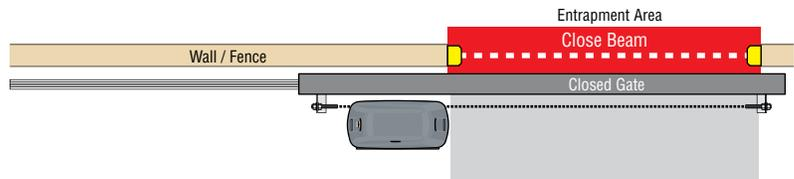
**3 OPEN Edge/Beam Reverse:** Obstructed reversing edge or photo beam will reverse the gate to the close position **during the opening-direction only**.
