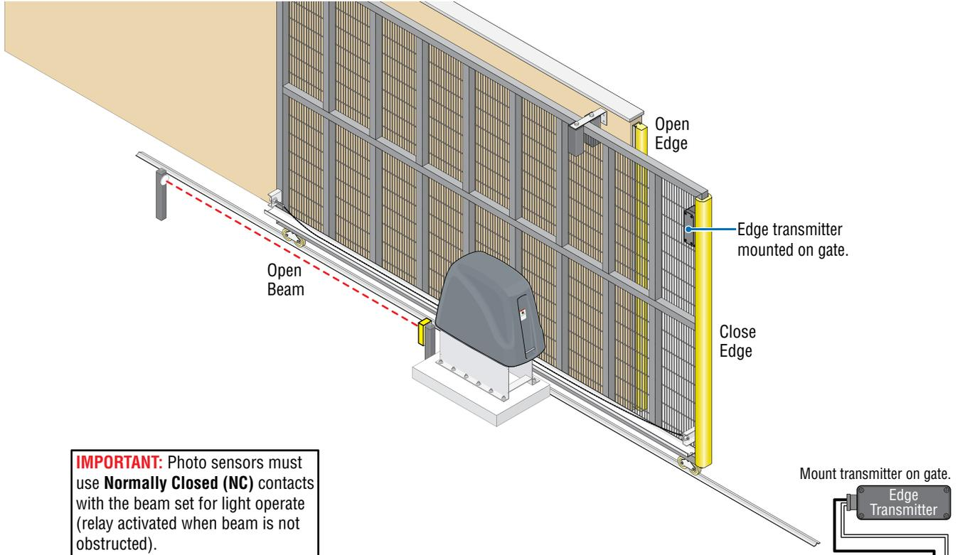
**IMPORTANT:** Photo sensors must use **Normally Closed (NC)** contacts with the beam set for light operate (relay activated when beam is not obstructed).
