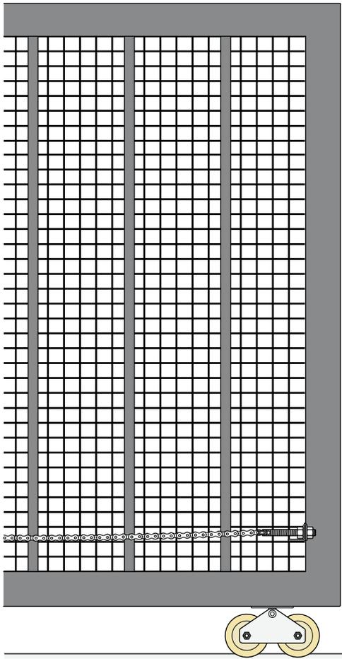
DoorKing recommends installing screened wire mesh on the **ENTIRE** gate **AND** on that portion of the adjacent fence that the gate covers in the open position. (See above).
