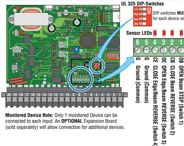
**Monitored Device Note:** Only 1 monitored Device can be connected to each input. An **OPTIONAL** Expansion Board (sold separately) will allow connection for additional devices.
