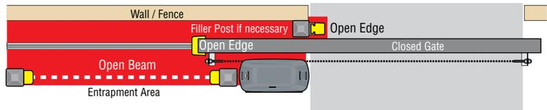
**4 CLOSE Edge/Beam Reverse:** Obstructed reversing edge or photo beam will reverse the gate to the open position **during the closing-direction only**.
